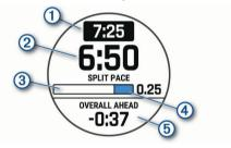
The device displays your target split pace ①, current split pace ②, completion progress for the split ③, distance remaining in the split ④, and overall time ahead or behind of your target pace ⑤.
