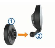
2 Open the lever ③, press the suction cup to the windshield, and flip the lever back toward the windshield.
