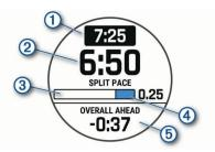
The device displays your target split pace (1), current split pace (2), completion progress for the split (3), distance remaining in the split (4), and overall time ahead or behind of your target pace (5).
